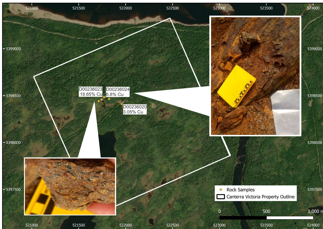
Figure 2. Rock grab samples at the Victoria Project (UTM NAD83 Zone 21N datum). Inset 1 and 2: Sample D00236020, outcrop grab sample with massive chalcopyrite and pyrite.
